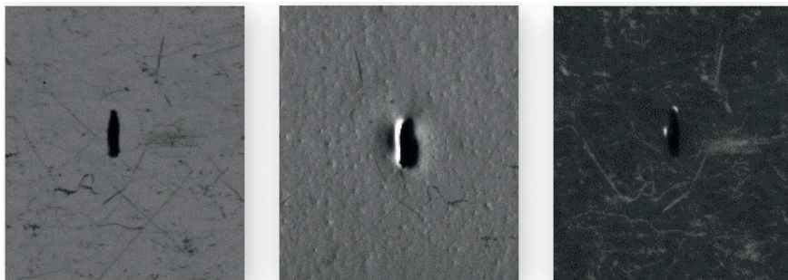
Fig. 1. Different lighting channels for example three channels: transmission bright field, transmission dark field (left, center) and reflection channel (right). © OCS
