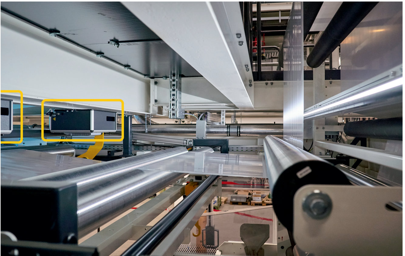
Film inspection system in a blown film line: the image processing systems detect surface defects such as gels, black specks, fish eyes, coating cracks, streaks, flow lines or insects. © OCS
